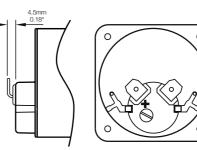
This is available as a rear mounted factory fitted option. The unit contains a Ø 6mm 'festoon' style lamp available in 6V, 12V or 24V. Please contact the sales office for more
