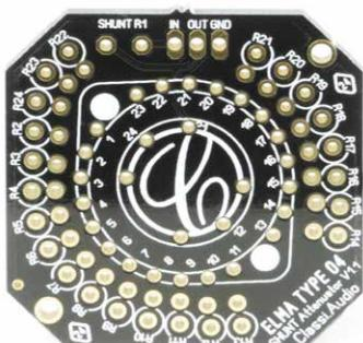
Only PCB SHUNT to Upgrade an Elma 04 Switch
